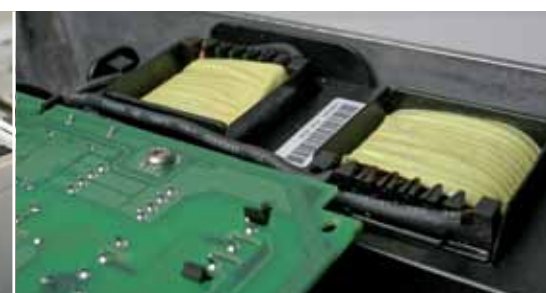
Built-in circuit chokes reduce the impact on the supply network and increase the lifetime of the drive.
