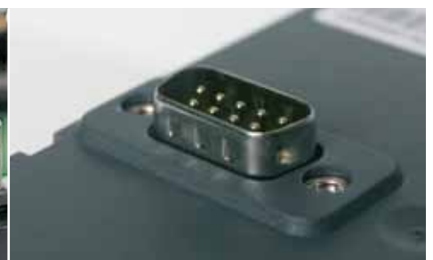
The VLT® AutomationDrive is controlled locally via a control panel. This is plugged in directly or connected via a cable to the robust Sub-D terminal – also while the drive is running.
